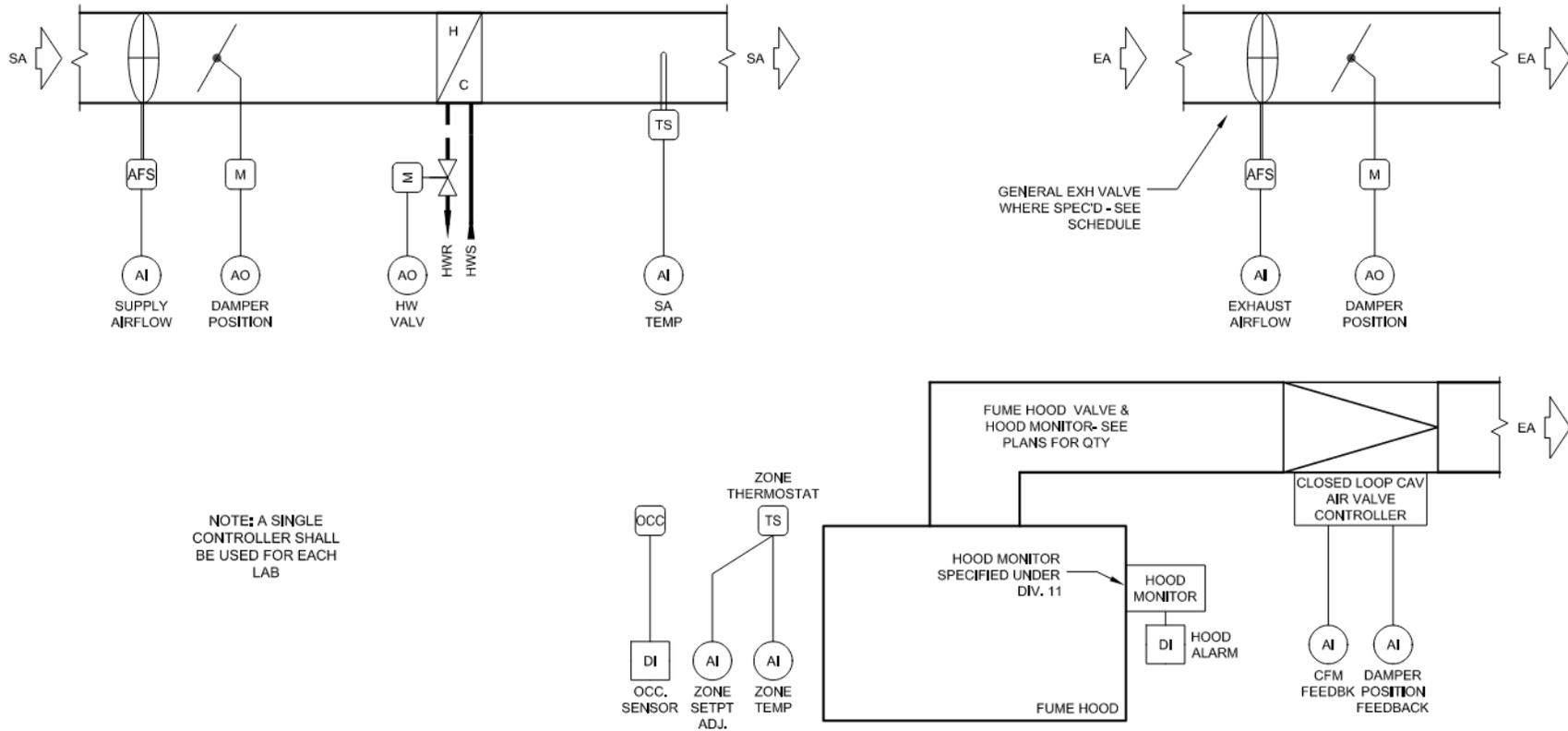
**A-32. Laboratory VAV Reheat Zone with Manufactured Venturi Air Valves**
