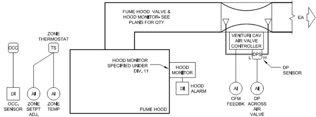
**A-30. Laboratory Four-Pipe VAV Zone with Manufactured Closed Loop Air Valves**
