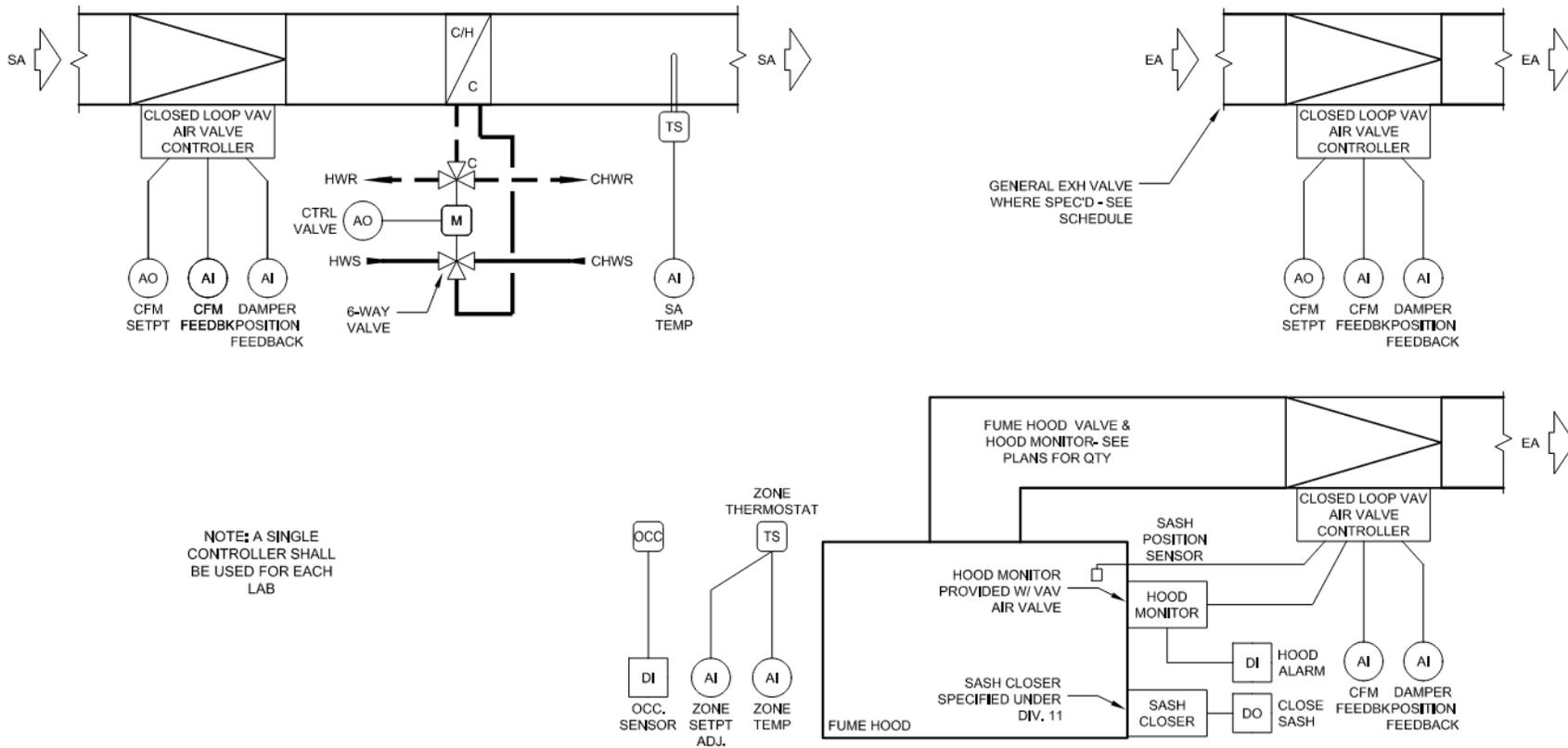
**A-31. Laboratory VAV Reheat Zone with Supply Air and General Exhaust Air VAV Boxes**
